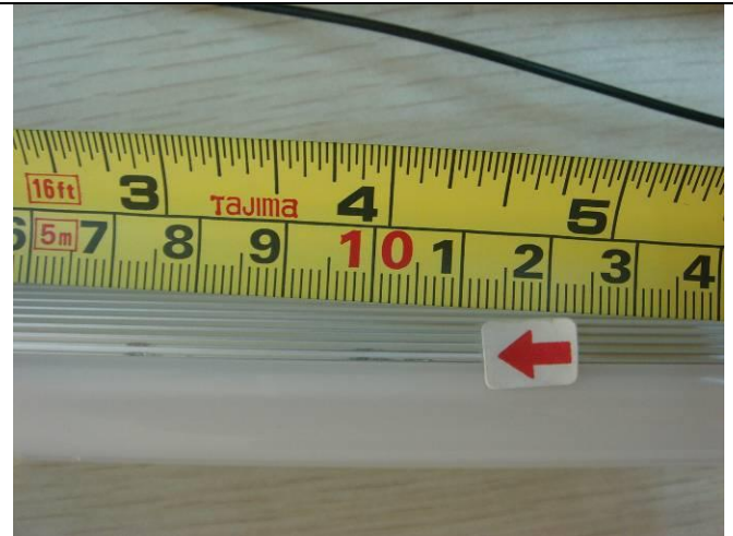
58. Minor defect: Scratch mark on unit (T8-60CM-10W)
