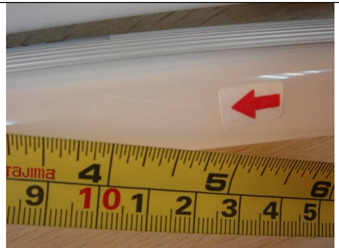
64. Minor defect: Scratch mark on unit (T8-150CM-25W)
