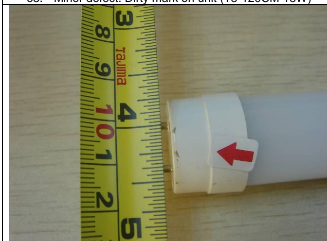
65. Minor defect: Dirty mark on unit (T8-150CM-25W)
