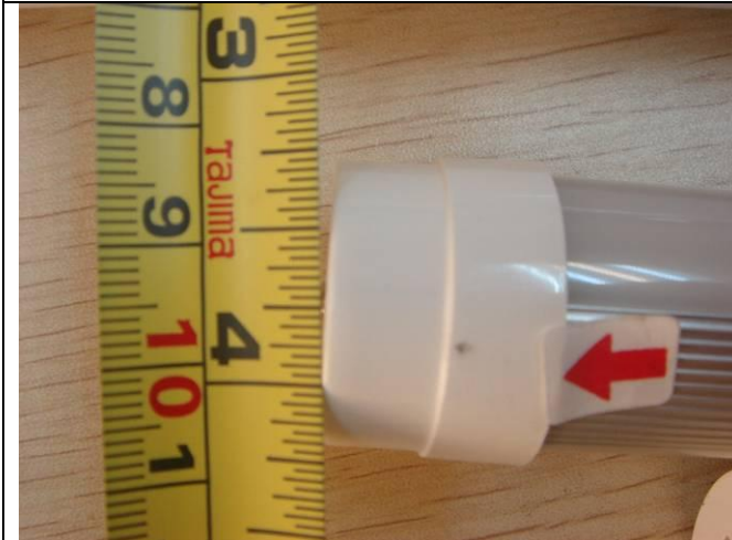
59. Minor defect: Dirty mark on unit (T8-60CM-10W)
