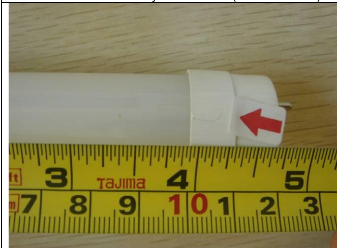
61. Major defect: Broken on one end of unit (T8-120CM-18W)
