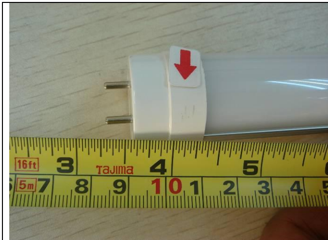
63. Minor defect: Dirty mark on unit (T8-120CM-18W)
