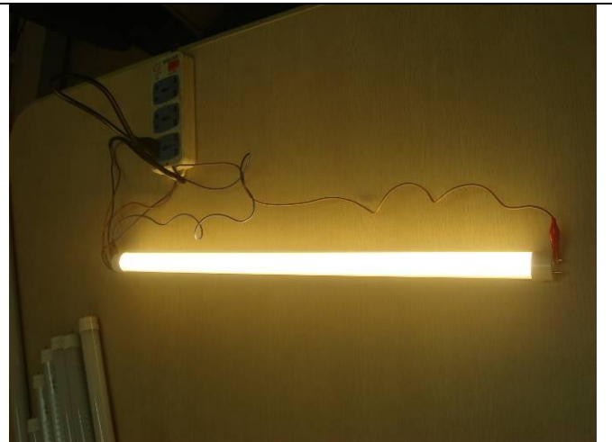
36. Low voltage running
