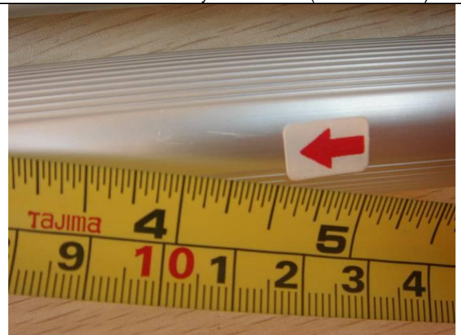
62. Minor defect: Scratch mark on unit (T8-120CM-18W)
